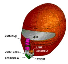
Racing EyeCue features a single-eye optical head-up display system with a reconfigurable color graphic presentation of vital racing data projected on a semi-transparent combiner. Conventional systems currently use a monochromatic fixed segment display.
